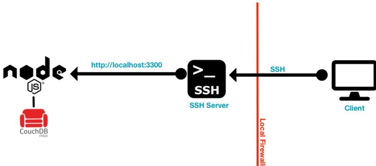
Ssh authentication is a special authentication method reserved exclusively for desktop clients. Ssh authentication first makes a direct ssh connection to the remote server. After the ssh connection successfully logs in, ssh then runs the fastx-protocol command which is used for communication between the ssh client and the FastX server. This connection is valid as long as the ssh connection stays up.
